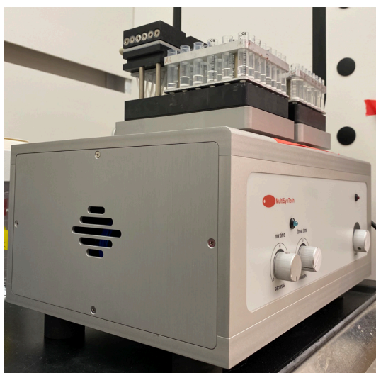
Figure 4. Vortex mixer with 2 U-Block Reactors mounted
